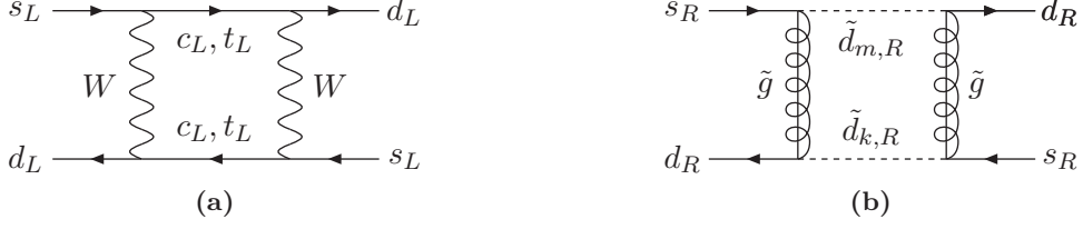
Figure 1. Dominant short-distance contributions to M_{12}^K (a) in the SM; (b) in the CMM extension.
